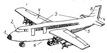
... cockpit ... fin ... fuselage ... hatch ... nose ... rudder ... undercarriage ... wing
